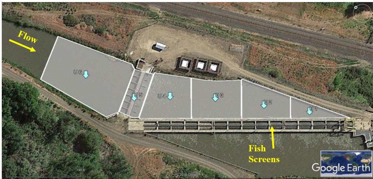
Figure D2-2. Delineated sections of the area upstream of the fish screens at Wapato Diversion (grey polygons and blue arrows). Sections U1, U2, U3, and U4 divide the area immediately upstream of fish screens. Section U5 surrounds the trashrack, and U6 is located in the upstream canal, reaching 50 m upstream of the trash racks (total upstream canal length is 780 m). Water flow is moving from left to right.
