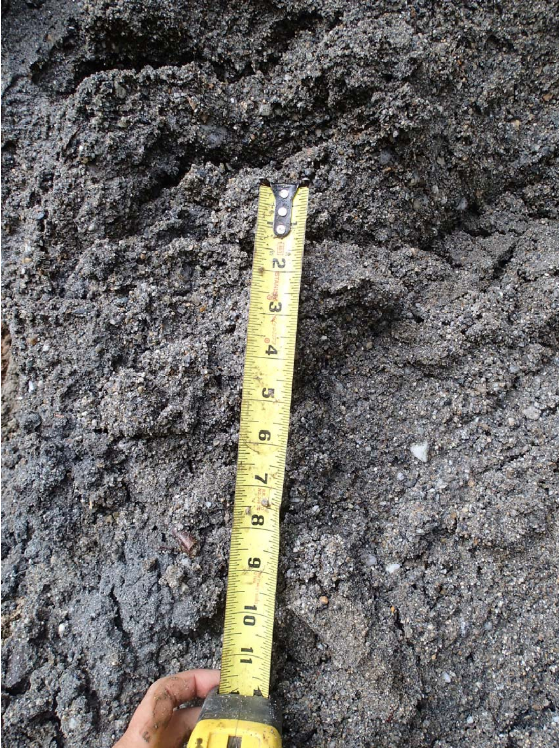
Figure 3 Non-cohesive sandy soils from Test Pit 2
