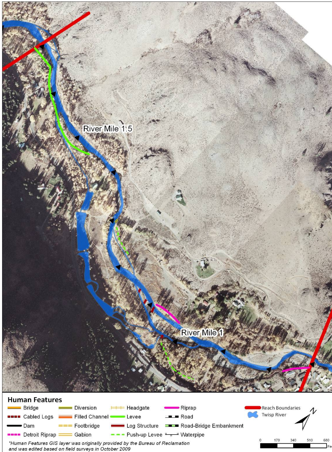
Figure 15. Aerial photo showing human features in Reach T2a. Flow is from west to east. Processes are hindered by bank hardening and development within the floodplain.
