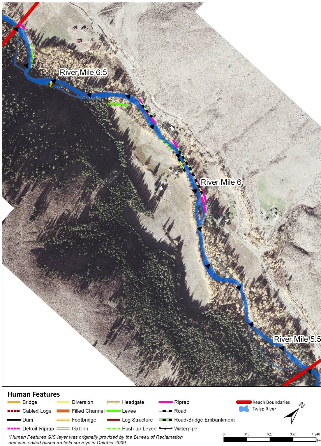
Figure 37. Aerial photo showing human features in Reach T3b. Flow is from west to east. Constraints include roads, a bridge crossing, bank hardening, and floodplain development.
