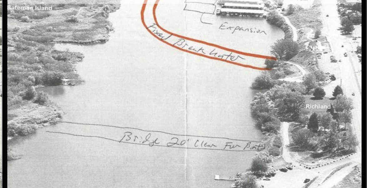
Alt. 8: Full breach & breakwater
