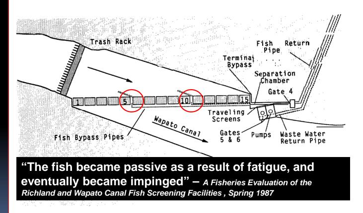
FIGURE 4. Flow Control Structure and Fish Bypass System in the Wapato Canal Fish Screening Facility Assuming uniform fish distribution above Sunnyside Dam, about 75% of the fish in the Yakima River may be diverted through the Sunnyside Canal Fish Screening Facility. - A FISHERIES EVALUATION OF THE SUNNYSIDE CANAL FISH SCREENING FACILITY, SPRING 1985
