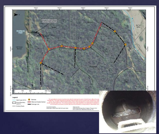
During dewatering, relative elevation along pipe changes
