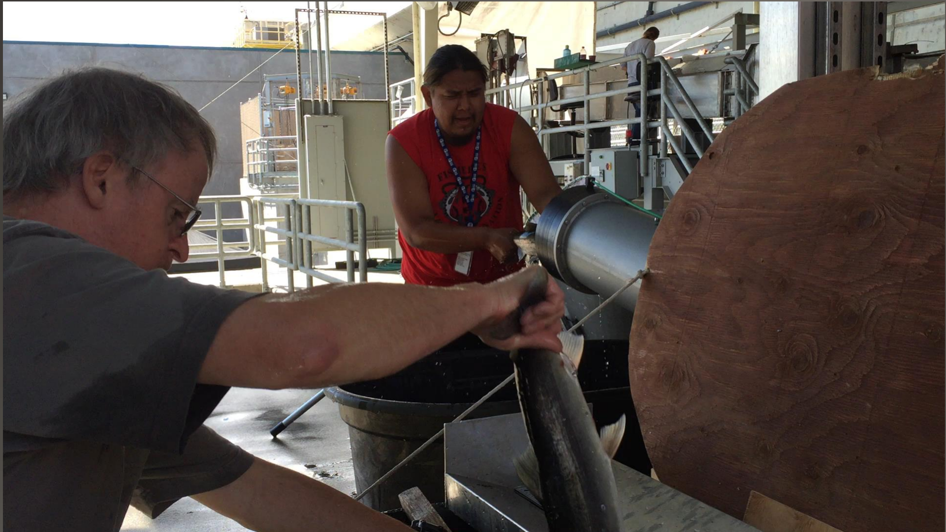
Jeff of CRITFC and Jim of YN sampling sockeye and loading into Whooshh system for 100 ft transport to calm water channel and continued passage up Priest Rapids fish ladder
