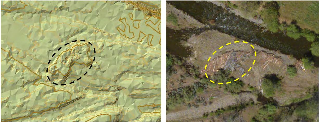
**Figure D3.** Example of woody debris raft causing a 2-3' high spot in the terrain model. Circled feature is likely reasonably stable to at least Q2. In the absence of stabilizing vegetation, it is likely mobile at Q25 and above. At discharges between Q2 and Q25, how to treat in a hydraulic model would depend on study objectives and would require discretion by the modeler.
