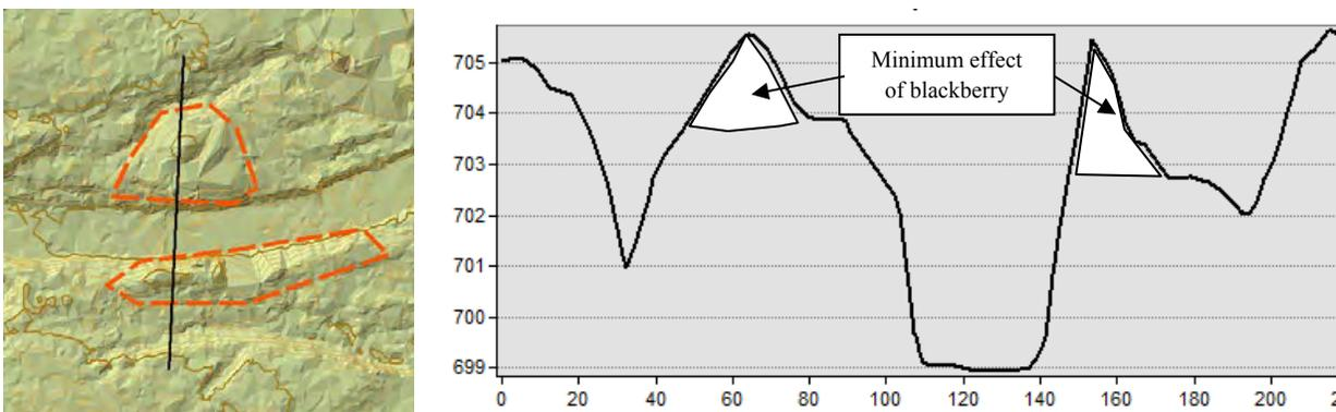
**Figure D5.** Example of blackberry effect on terrain model (left) on cross-section (right) has implications for hydraulic modeling.
