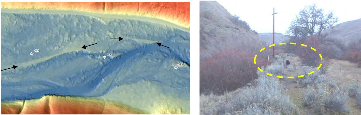
**Figure 26. Remnants of the mid-valley, pre-1964 flood alignment of the Rock Creek Road persist 1-4' above adjacent topography for approximately 1300 lineal feet; vicinity VM 10.4.**
