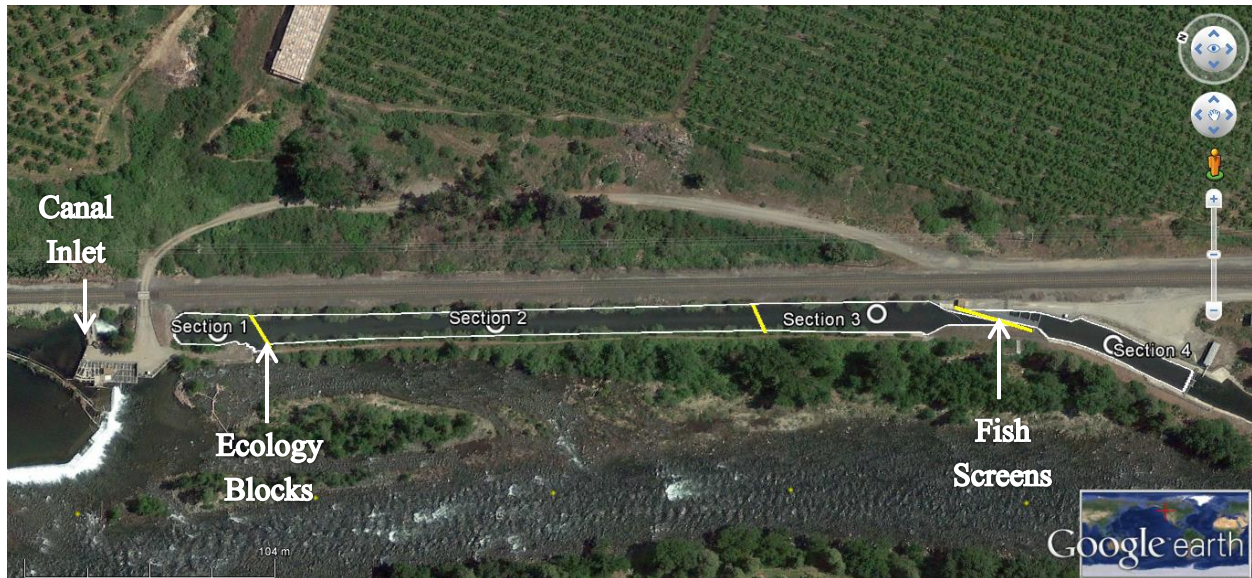
Figure G8-1. An overview map showing the four sections of Dryden Diversion.
