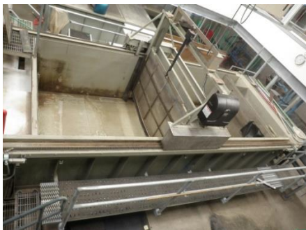
Figure G3-10. Subsampling holding pool overview (from side). The crowder has a 2.2 mm mesh opening. At the downstream end of the holding pool, there were some 9.5 mm gaps that lead to a dead end opening.
