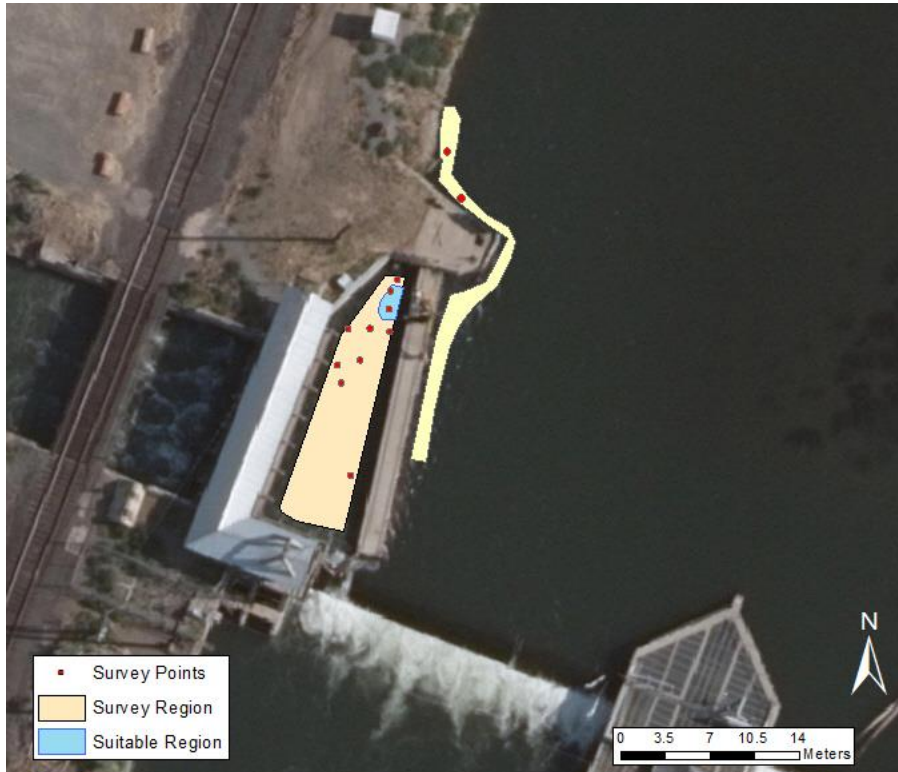
Figure G4-5. Wapato headgate region illustrating total survey region (yellow and blue polygons) and suitable region (blue polygons) from surveys conducted on October 15, 2015.
