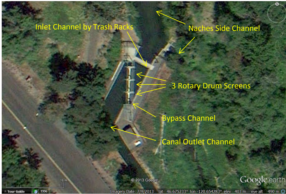
Figure 1. An aerial map of Congdon Diversion with labels for key components.
