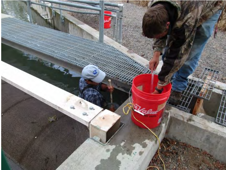
Figure 6. Releasing 0+ age Pacific lamprey larvae 1 m in front of the bypass net at the bottom of the water column to test trap efficiency.
