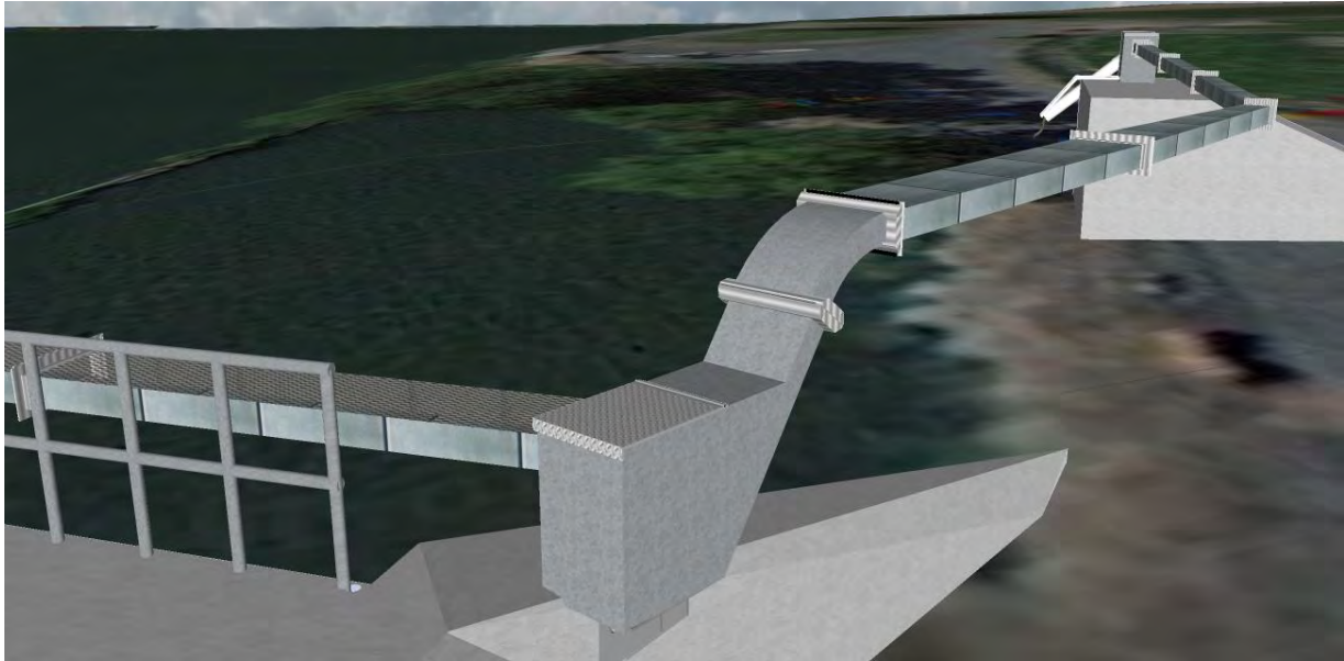
Figure 17. The Third section for the proposed LPS on the left bank at Prosser Dam, showing the rest box and flume extending upstream to the upwell box.
