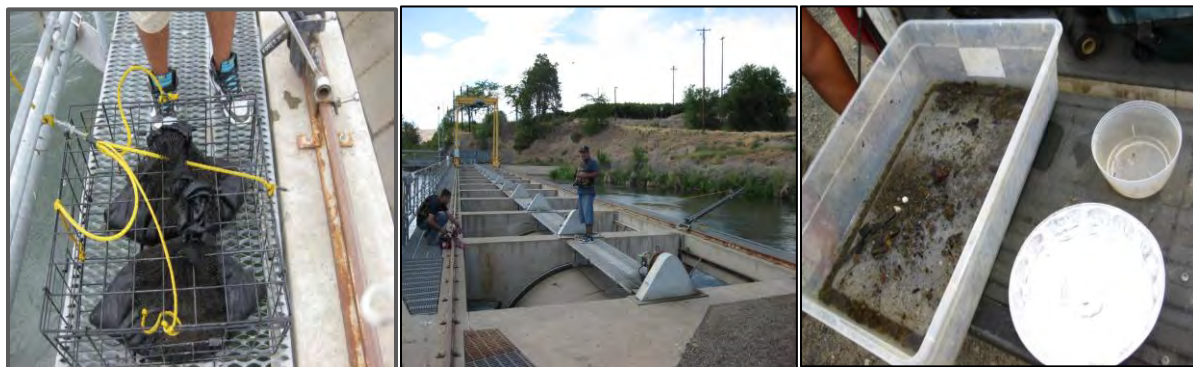
Figure 3: Pictures of an assembled sediment trap from June 2013 (left); operating the boom and winch to pull the trap up from the downstream side of the rotary drum screens at Sunnyside Diversion (middle); and sieved material, ready for sorting and identification (right).
