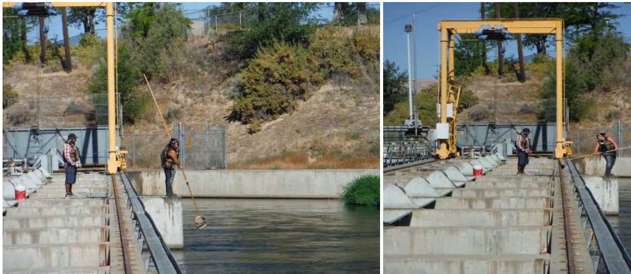
Figure 8: Yakama Nation staff using the modified D-frame kick net (Left). Lowering the length of the pole to sweep towards the structure and quickly pull up and out of the water to turn the net out into a plastic tub on the structure (Right).
