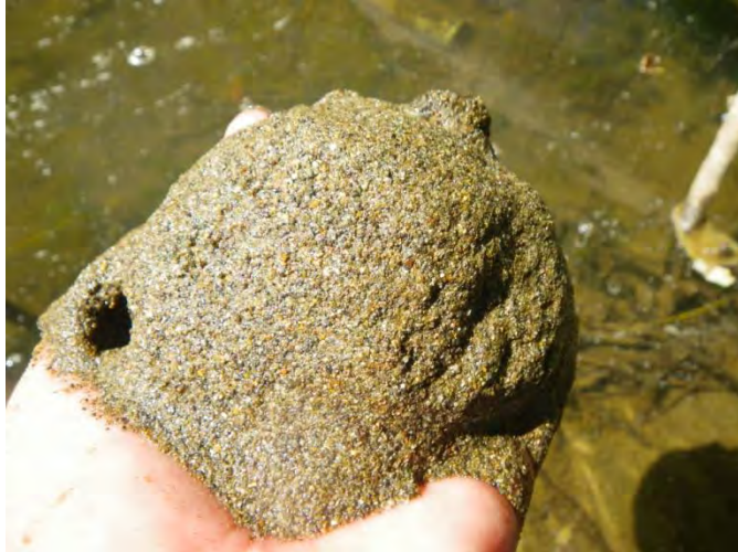
RK246.9: Close up of the sediment that was composed of sand mixed with small amounts of silt
