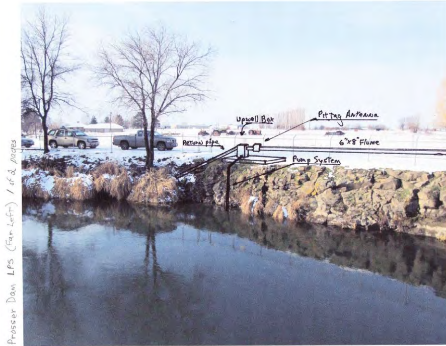
Figure 9. A photo with an engineer drawing depicting the proposed route on the far left LPS site at Prosser Dam (the upstream half). The specific route and dimensions can certainly be modified, but it provides one example of what the LPS would look like.
