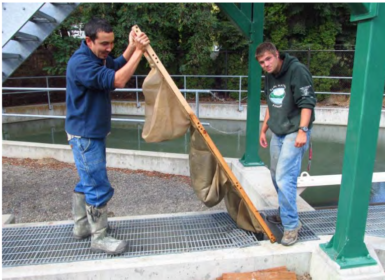
Figure 5. Inserting a custom made net for the trap efficiency test in the bypass channel.
