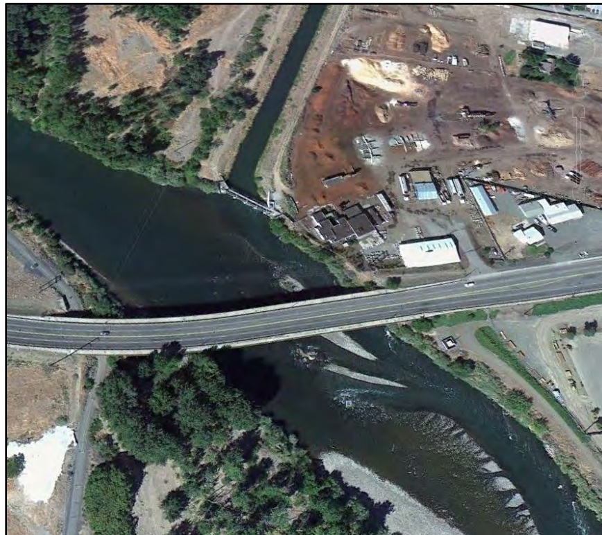
Figure 19. Aerial photo showing the gravel bar and thalweg of the Yakima River at the Roza Wasteway #2 confluence.
