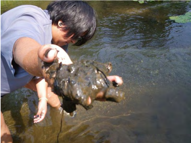
NA15: Markeyta Pinkham holding sediment for a close up, this area was composed of soft silt mixed with small amounts of woody debris
