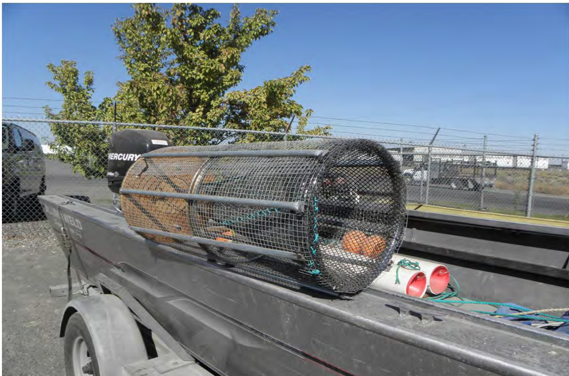
Figure 2. Bicycle lamprey trap.
