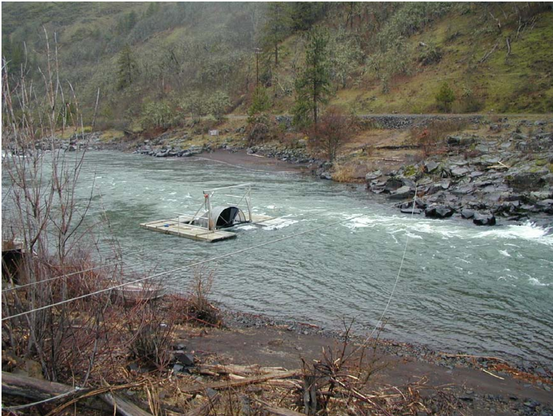
Figure 6. Rotary screw trap at river kilometer 4 on the Klickitat River.
