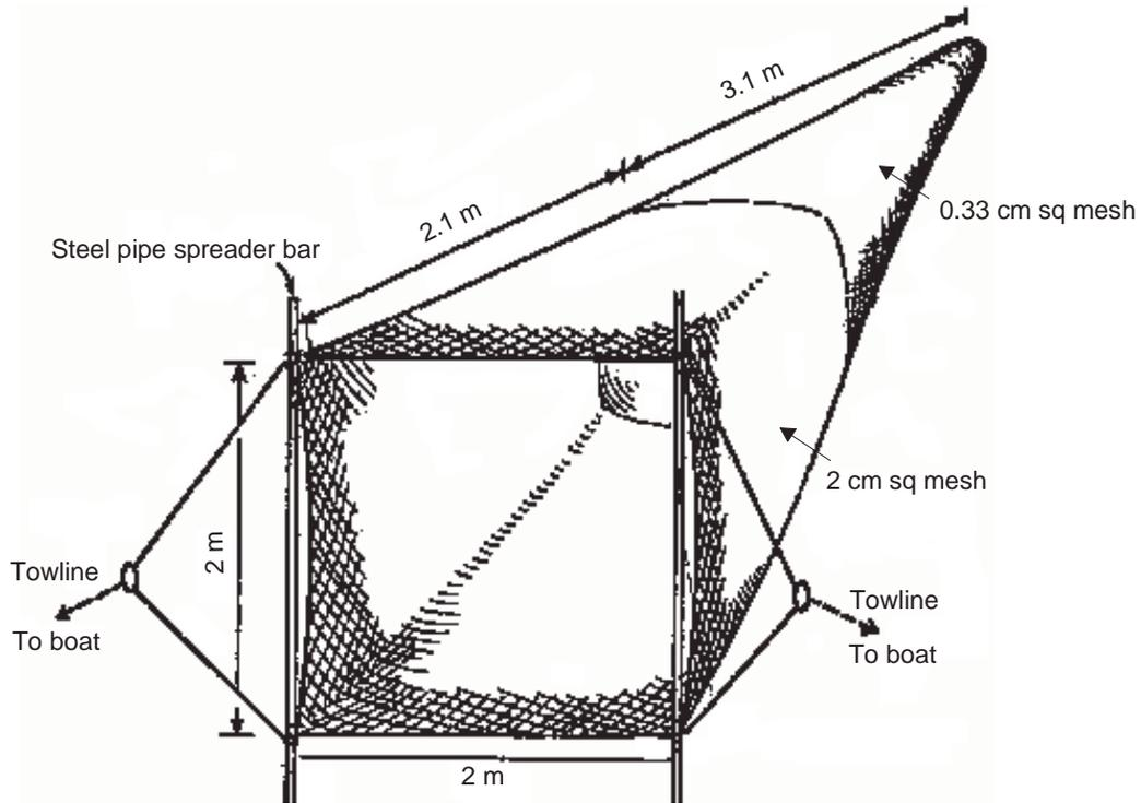
Figure 4. Diagram of tow net used in 2002.
