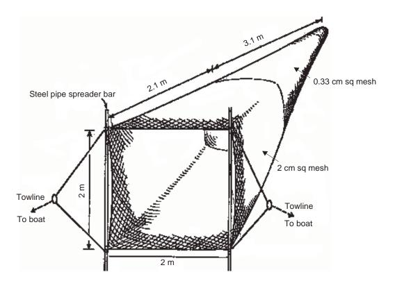
Figure 4. Diagram of tow net used in 2002.
