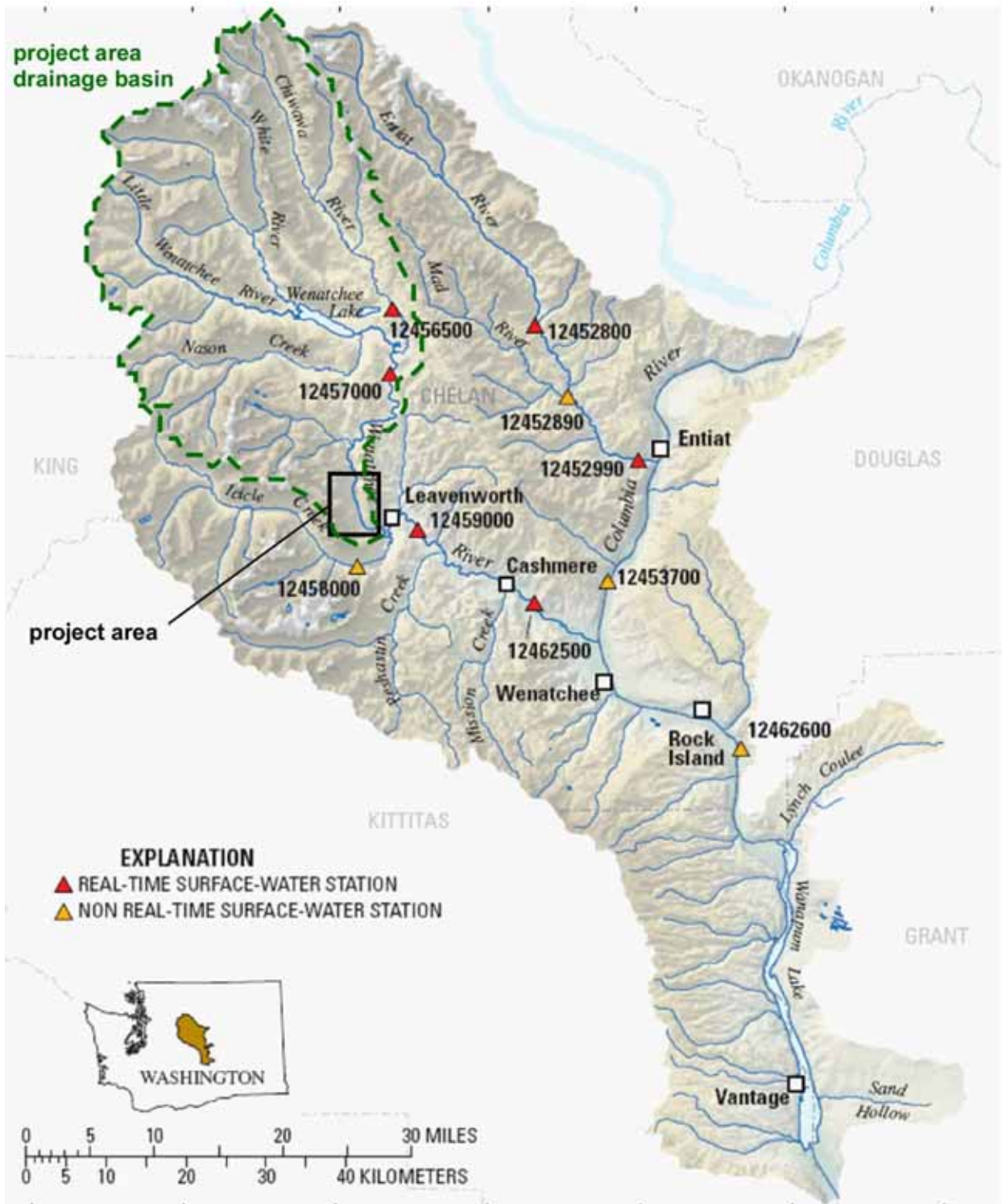
Figure 4-1. Project Reach Drainage Area in the Wenatchee River Basin and Gaging Stations.
