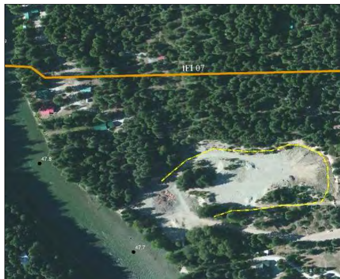
Figure 67. Gravel excavation pit (highlighted in yellow) along left bank in upstream portion of Reach 6.
