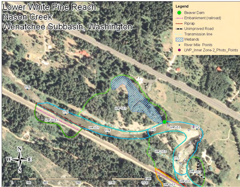
Figure 1. A plan view showing the upstream end of the Lower White Pine reach with the location of LWP IZ-2, photo points, location of anthropogenic features, and the proximity of adjacent subreaches with the corresponding restoration strategies.
