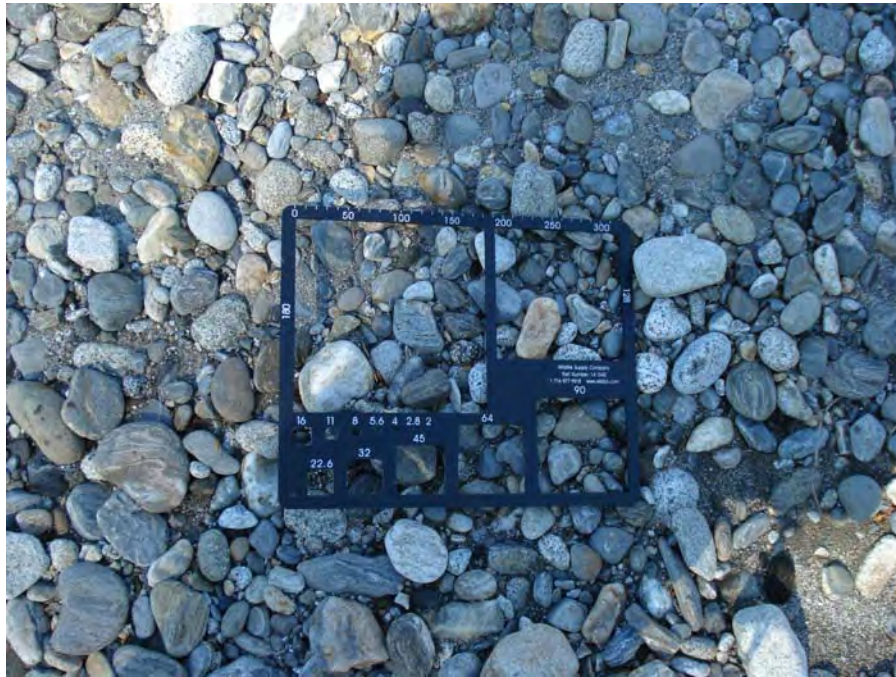
Photograph No. 10. View showing the material on the gravel bar with the gravelometer for scale. Lower White Pine Reach; Subreach IZ-4, Nason Creek - Wenatchee Subbasin, Washington. Bureau of Reclamation Photograph by R. McAfee; May 5, 2007.
