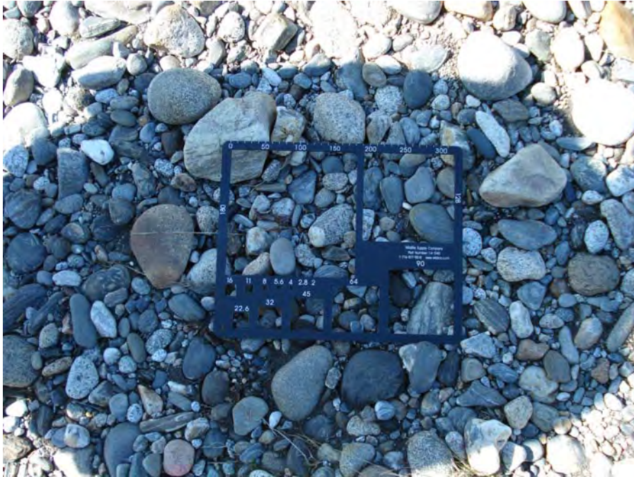
Photograph No. 7. View of the material on the gravel bar with gravelometer for scale. Lower White Pine Reach; Subreach IZ-3, Nason Creek - Wenatchee Subbasin, Washington. Bureau of Reclamation Photograph by R. McAfee; May 5, 2007.
