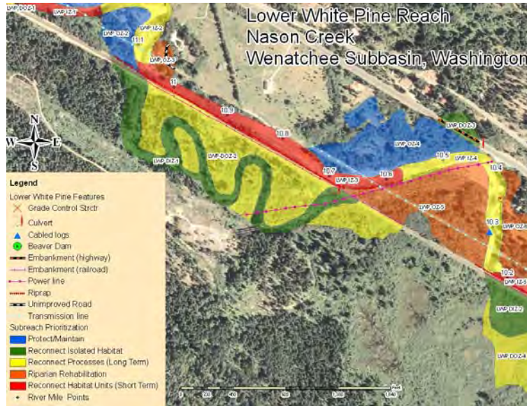
Figure 50 - A plan view showing the location of LWP IZ-3 in the downstream end of the Lower White Pine reach, location of anthropogenic features, and the proximity of adjacent subreaches with the corresponding rehabilitation strategies.
