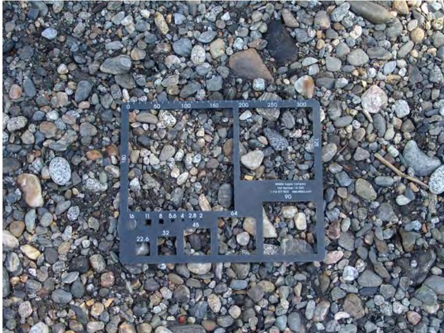
Photograph No. 2. View is of material on the gravel bar with gravelometer for scale. Lower White Pine Reach; Subreach IZ-3, Nason Creek - Wenatchee Subbasin, Washington. Bureau of Reclamation Photograph by D. Bennett; August 8, 2007.
