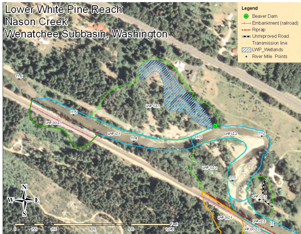
Figure 1. A plan view showing the upstream end of the Lower White Pine reach with the location of LWP OZ-1 location of anthropogenic features, and the proximity of adjacent subreaches.
