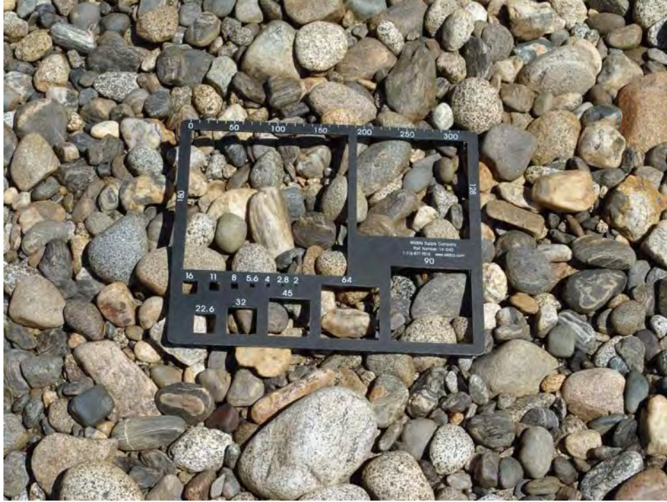
Photograph No. 4. View of material on gravel bar with gravelometer for scale. Lower White Pine Reach; Subreach IZ-6, Nason Creek - Wenatchee Subbasin, Washington. Bureau of Reclamation Photograph by D. Bennett; August 8, 2007.
