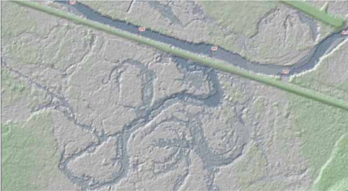
Figure 23. Example of disconnected historical channels and floodplain between RM 9.6 to RM 9.9. Colors represent elevations relative to present main channel elevations, dark blue being the closest and green being the farthest (highest elevations). The railroad embankment can be seen in green running along the present channel identified by red river mile markers, flowing from upper left to right in the image.
