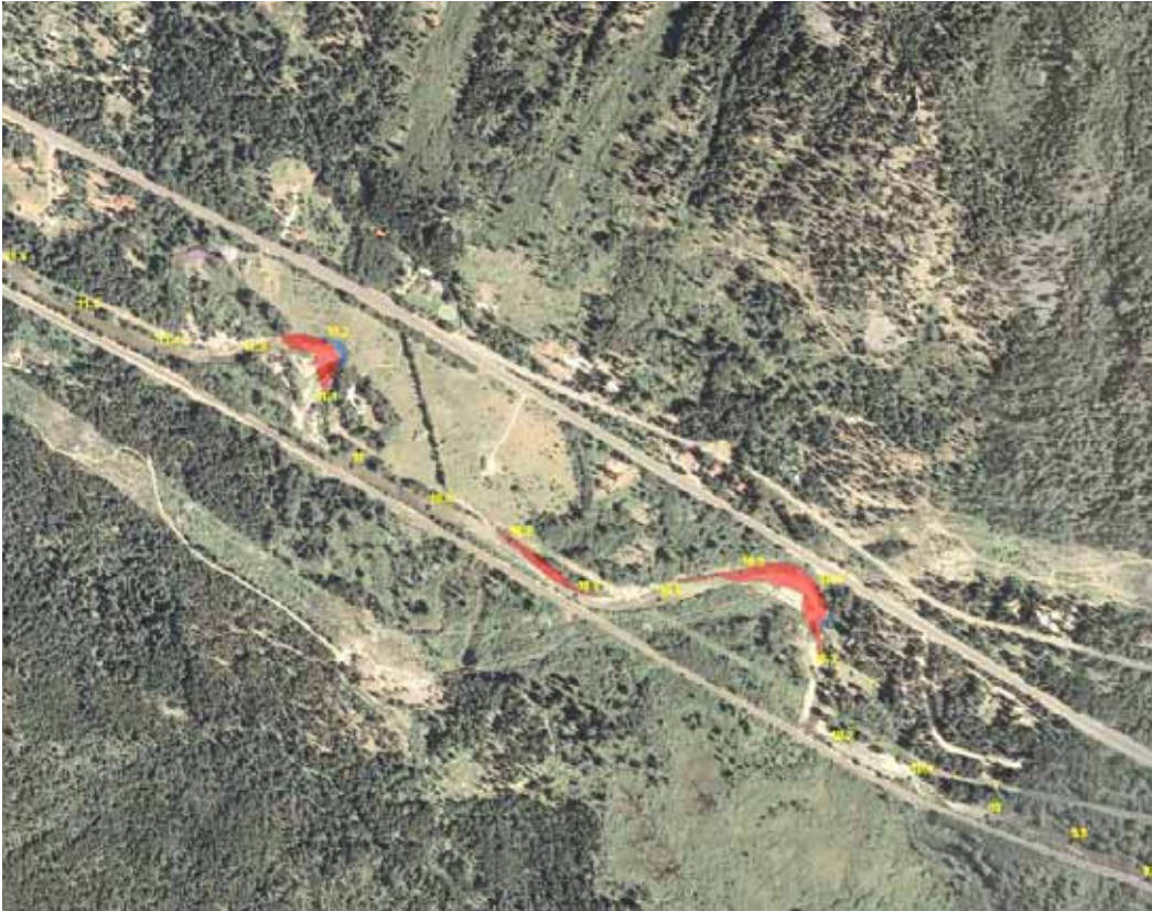
Figure 33. Example of two meandering channel locations (between artificially confined sections) where bank erosion along the outside of a meander bend at RM 10.4 and 11.2 occurred between 1962 and 2006 (colored polygons show erosion areas) (also see maps 29 and 30 in atlas for more locations of channel areas that have been reworked).
