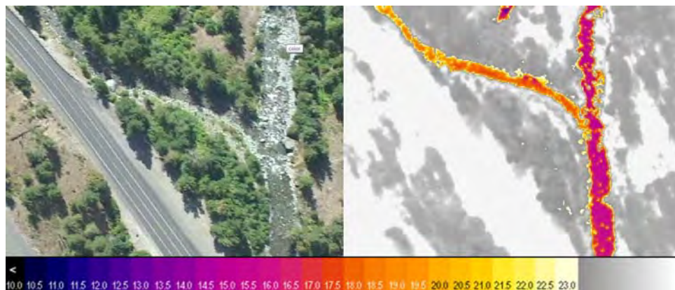
Figure 53. Thermal (TIR) image of Peshastin Creek at the Ingalls Creek confluence. The temperature scale at the bottom is in degrees Celsius. Streamflow is from top to bottom of images. Ingalls Creek enters at the top right and upper Peshastin is at left. Ingalls Creek is an important contributor of cool water to Peshastin Creek, and its impact carries downstream for a few miles.
