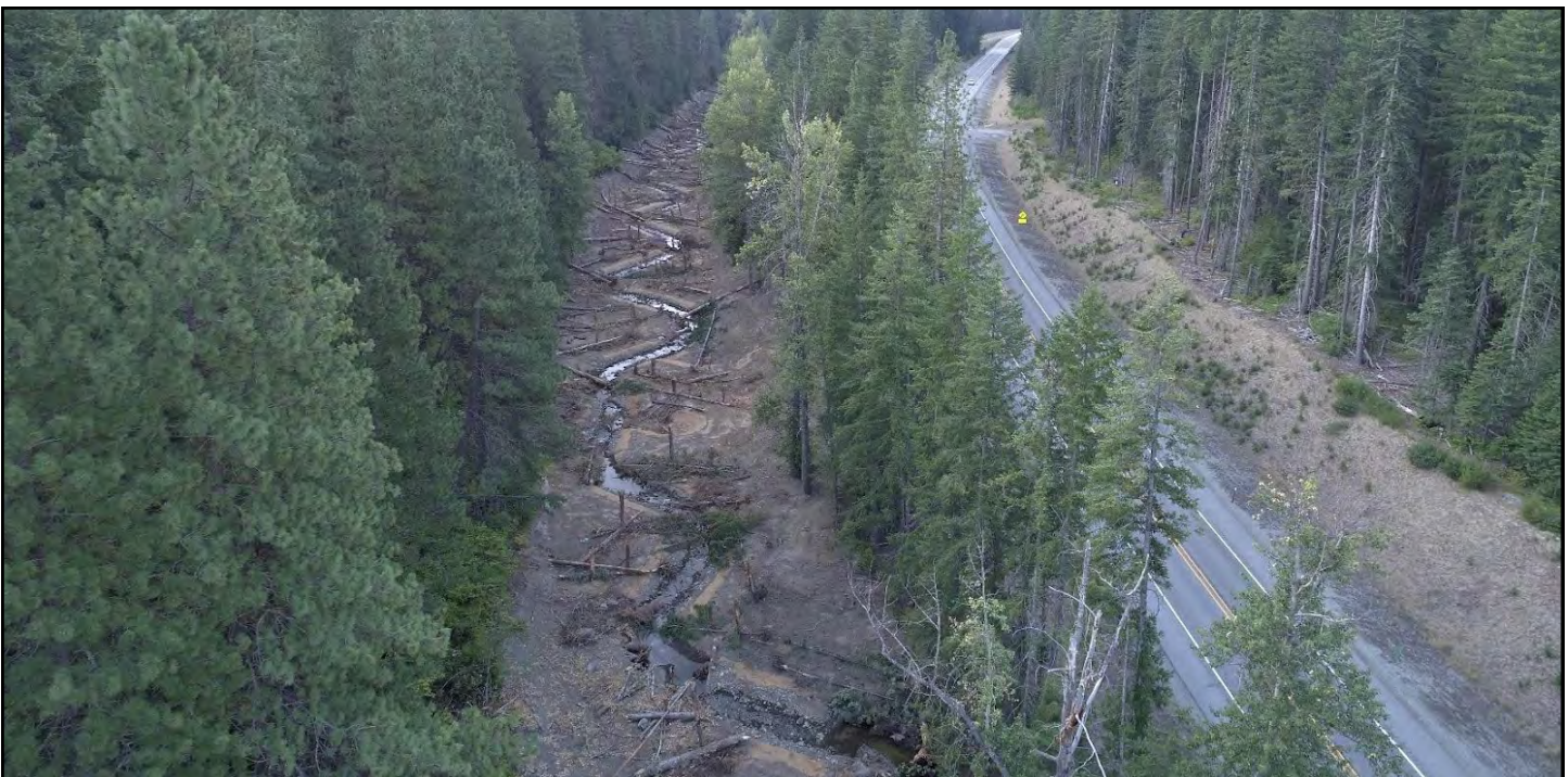
Reconstructed 0.4 mile stream channel and floodplain habitat associated with Skinney Creek (YN)
