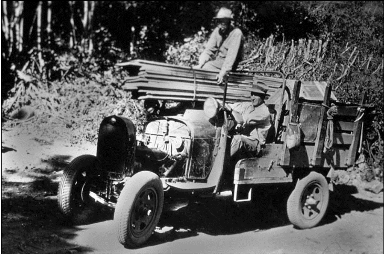
Figure 6. The Flying Cloud puddlejumper truck hauls lumber, probably towards the Azurite Mine, date unknown. In the early 1930s, three Model T trucks nicknamed puddlejumper were altered in Twisp. A vehicle was needed that could be driven from Robinson Creek, around Dead Horse Point and on to the Azurite Mine up and over the extremely narrow Hart's Pass. The front axle was narrowed by 12 inches and the rear axle replaced with one that allowed the trucks to gear down. An extra water tank, and an oil pump to lubricate the front bearing were also added. Ernie Cotton Collection, courtesy of the Shafer Museum and the Methow Grist Archive.
