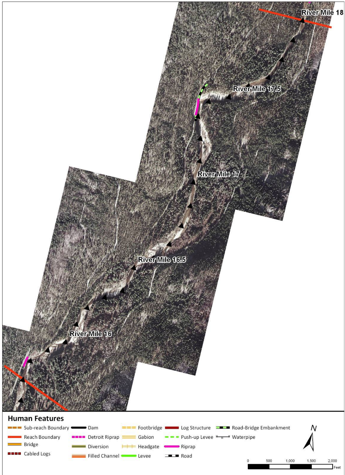
Figure 44. Aerial photo showing human features in Reach C8. Flow north to south.
