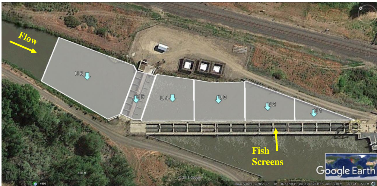
Figure 2. Delineated sections of the zone upstream of the fish screens at Wapato Diversion (light grey polygons and blue arrows). Sections U1, U2, U3, and U4 divide the zone immediately upstream of fish screens. Section U5 surrounds the trashrack, and U6 is located in the upstream canal, reaching 50 m upstream of the trash racks (total upstream canal length is 780 m). Water flow is moving from left to right.
