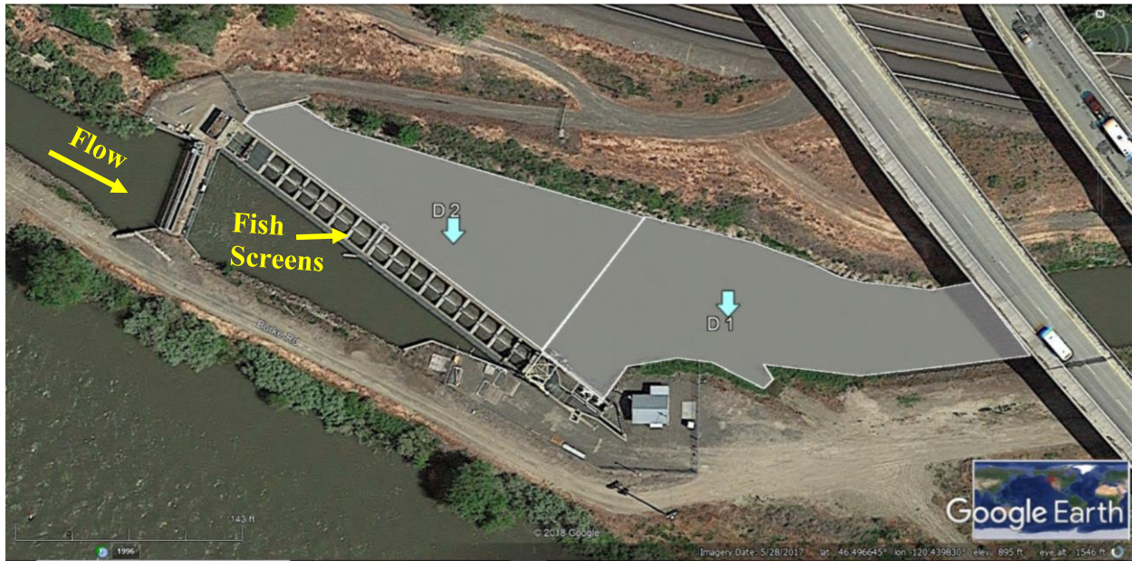
Figure 1. Delineated sections of the zone downstream of the fish screens at Sunnyside Diversion (light grey polygons and blue arrows). Section D2 is located immediately downstream of the fish screens, and Section D1 is located downstream of section D2, extending downstream to the I-82 Highway Bridge. Water flow is moving from left to right.
