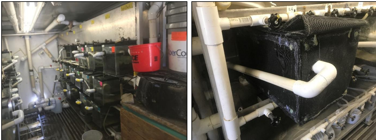
Figure 1. The overall aquaria set-up inside Prosser Fish Hatchery lamprey conex building where lamprey were monitored daily (left photo). The removable black mesh we used to cover the tanks and to keep them dark is also displayed (right photo).
