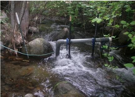
Figure 26. Instream PIT tag detection antenna in Lower Libby Creek at RM 0.3 (September 2011).
