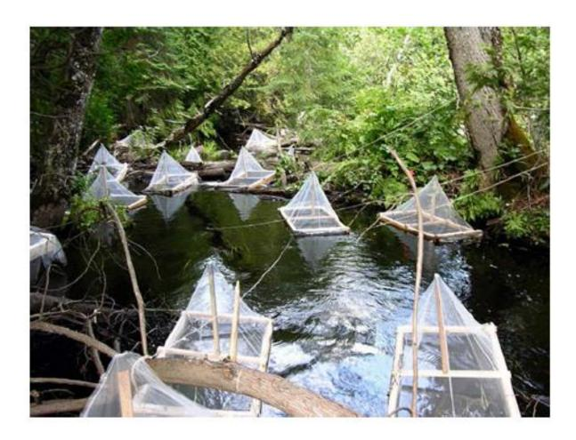
Fig. 1 Emergence traps used to sample aquatic insects emerging as adults. Each frame is 1 m  $\times$  0.5 m
