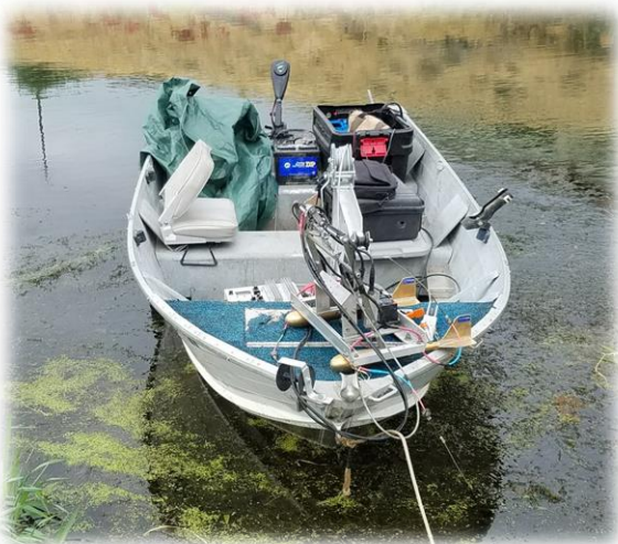
Photo L2. Survey boat (4 m V-hulled fishing boat) used to deploy the deepwater electrofishing platform at Sunnyside Screens.
