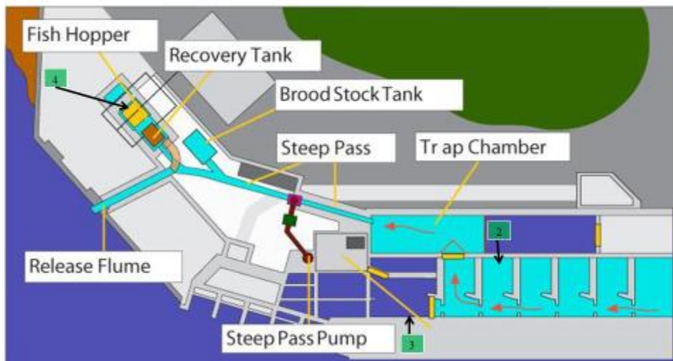
Figure 5. Diagram of the Upper portion of the Tumwater Dam Ladder showing the fish ladder as well as the trapping route. The three upper release locations are also shown (#s in green squares: 2, 3, and 4).
