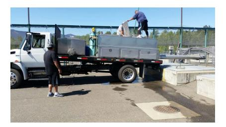
The Yakima Klickitat Fisheries Project received the new adult transfer truck and put it to use transferring adults from the 2015 brood. The truck has two tanks and a hydraulic bed that make fish release easy.
