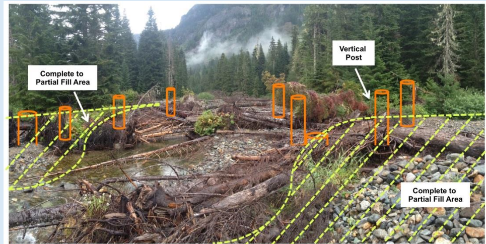
Proposed roughened floodplain concept
