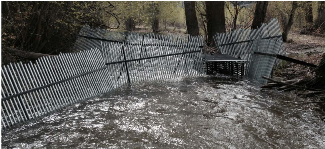
Figure 2.2 - Beaver Creek weir trap.
