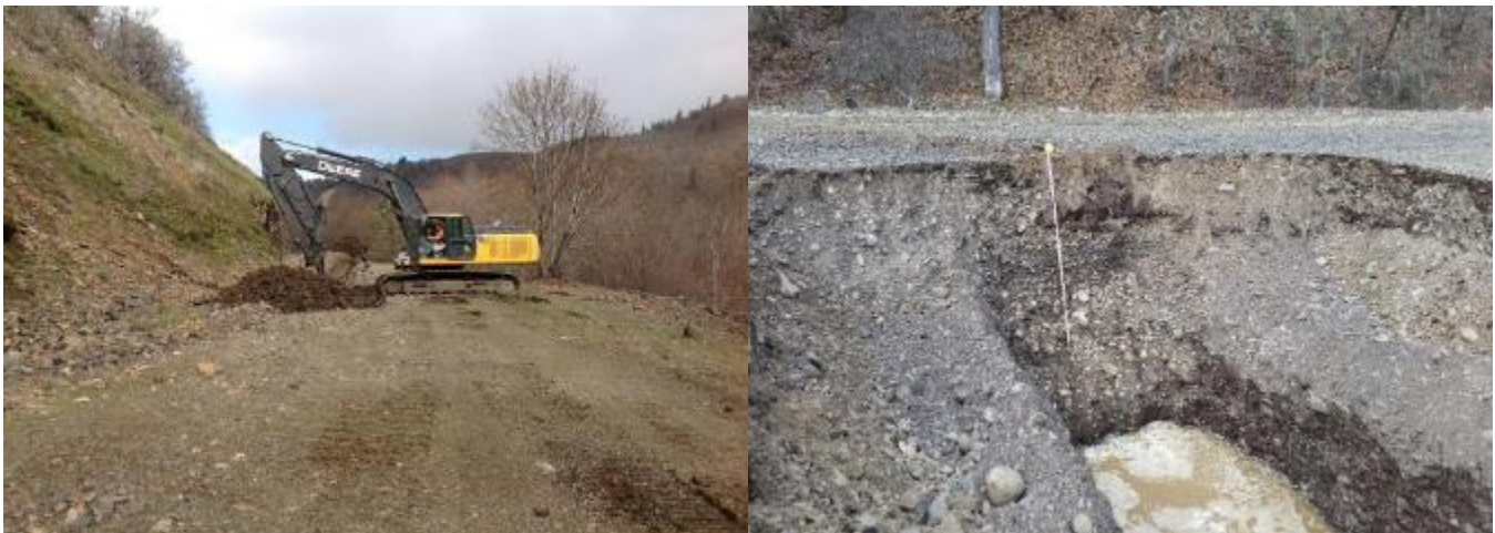
Figure 6. Example of test trench (left) and profile (right) displaying mixed alluvium fill and native soils.
