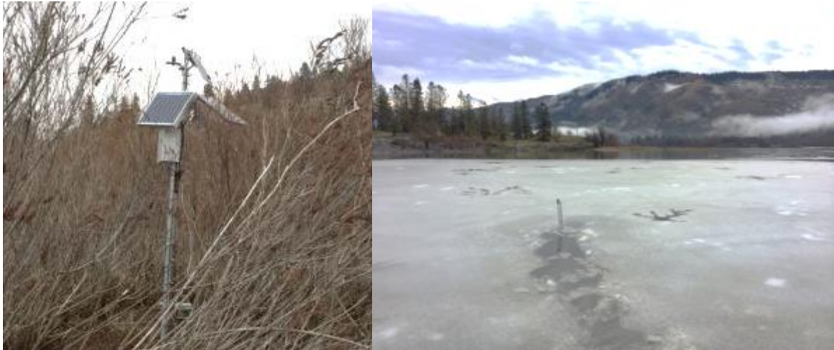
Figure 21. Mast and three-solar-panel array at East Delta (left) and February icing conditions.
