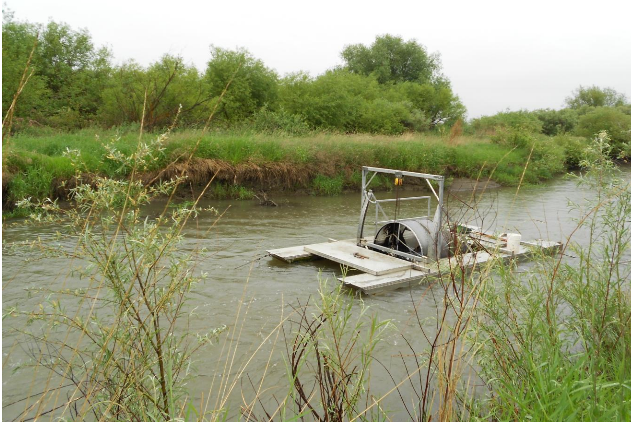
Figure A-1. Photograph of the 5-foot rotary screw trap at the upper Toppenish location (RM 26.5) including modifications.
