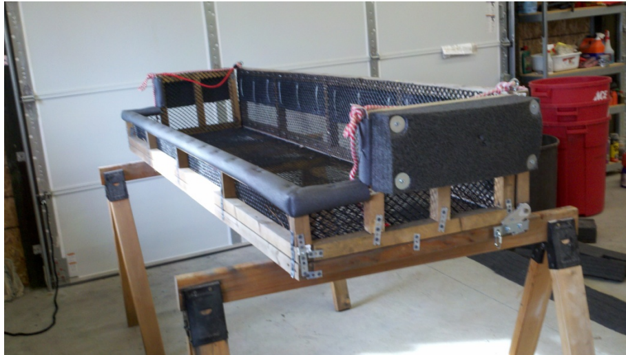
Figure 4.4 - Side view of trap with modified floatation and attachment.
