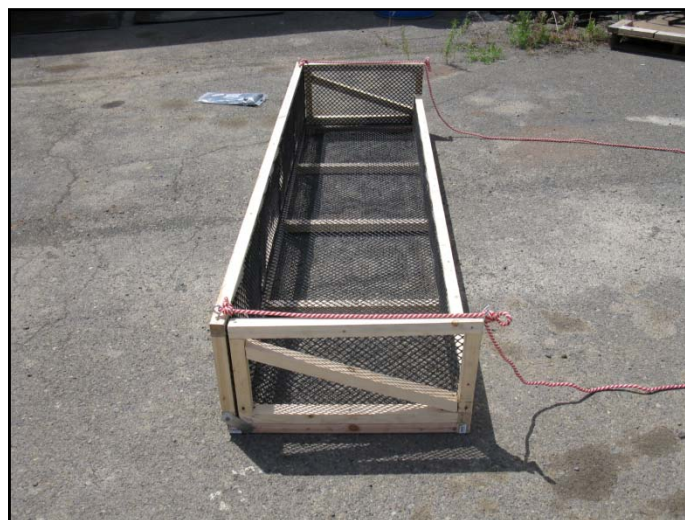
Figure 4.2 - Top view of prototype trap box for Twisp River steelhead kelt trap.
