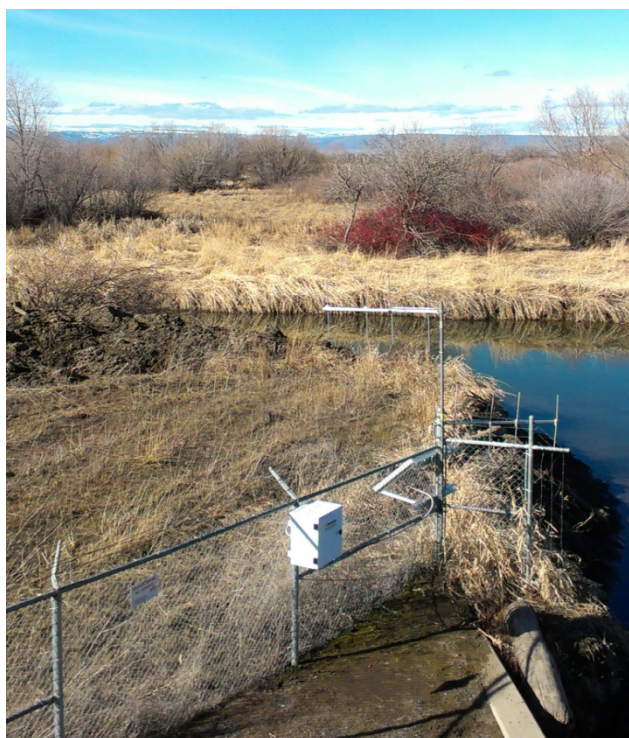
Figure 5. Typical Solar powered fixed site with two Yagi directional antennas positioned for upstream and downstream detections, upper Toppenish Cr.
