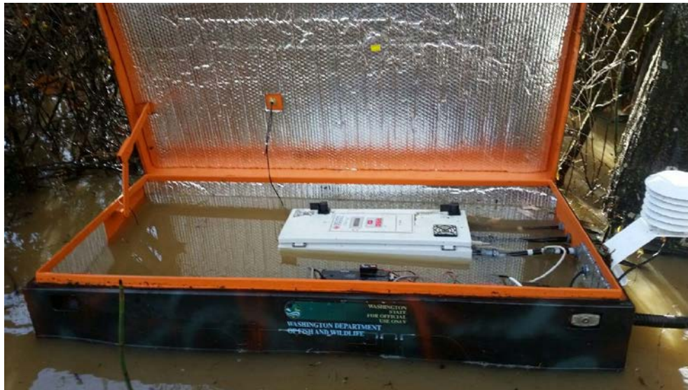
Figure 4. Lower Mainstem Teanaway River instream PIT tag detection equipment following a December 2015 flooding event.
