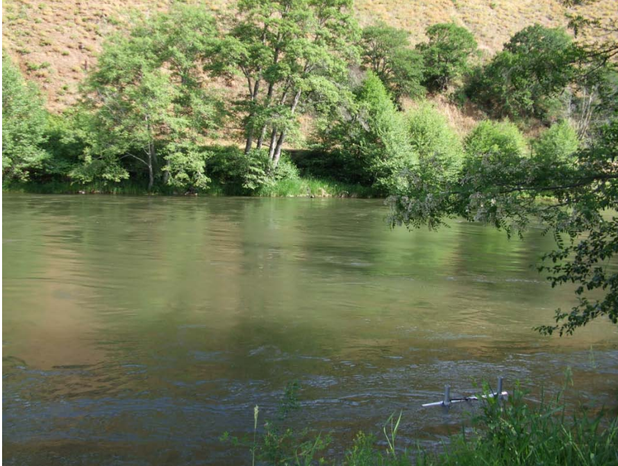
Figure 2. Transducer mount (lower right) deployed in the Klickitat River (RM 3.0), June 4-5, 2009. River discharge is approximately 2700 cfs, and some surface turbulence is evident at this level of discharge.
