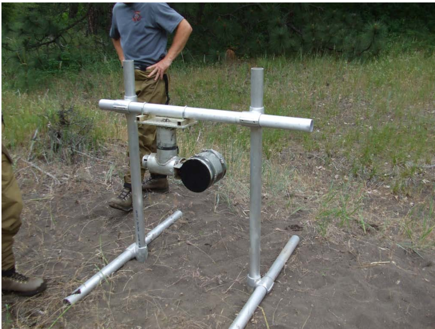
Figure 3. Transducer and dual-axis rotator attached to the transducer mount prior to deployment, June 4-5, 2009.
