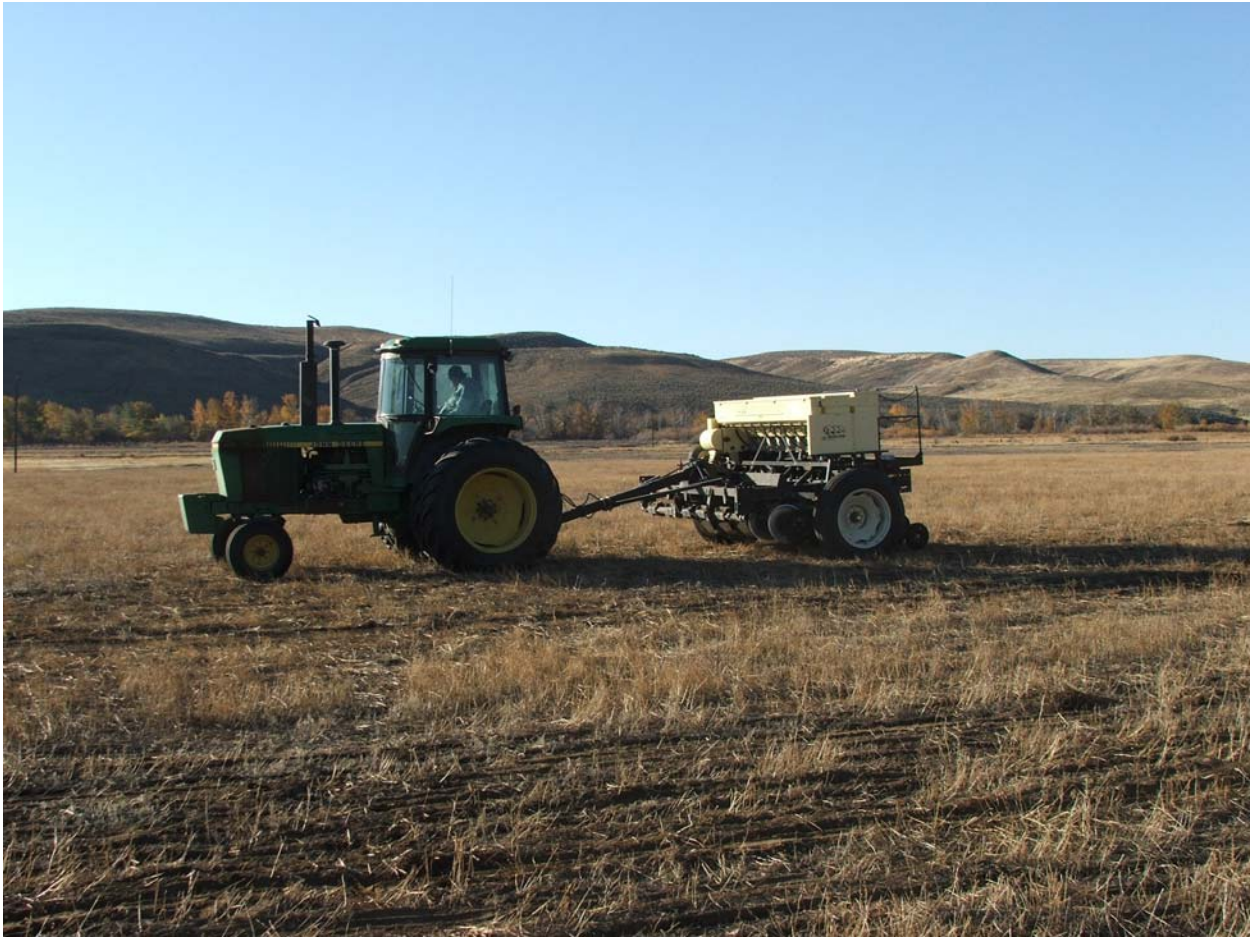
Seeding native grasses at Lower Satus (Tule Road 1) in October 2006. The no-till drill is effective at cutting through cheatgrass thatch and increasing seed-soil contact.
