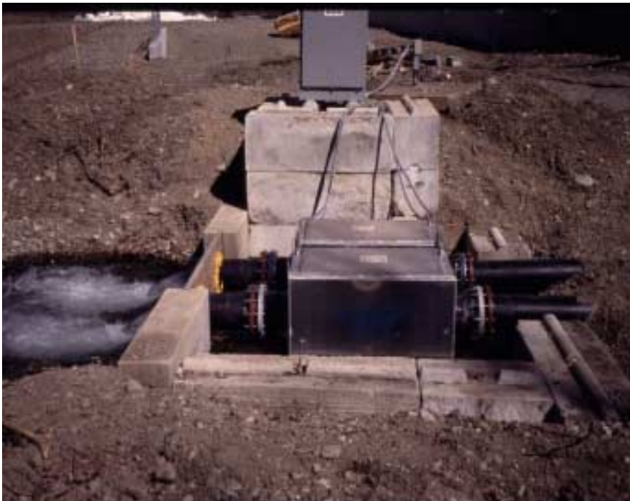
Figure 22. Spring chinook smolts with PIT tags are interrogated as they exit from their respective acclimation sites (Easton, N.F.Teanaway and Clark Flat).
