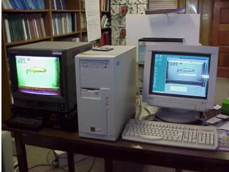
Figure 31. Shows the adult fish video monitoring video editor (Phase II), designed to capture and store to the PC harddisk target fish.
