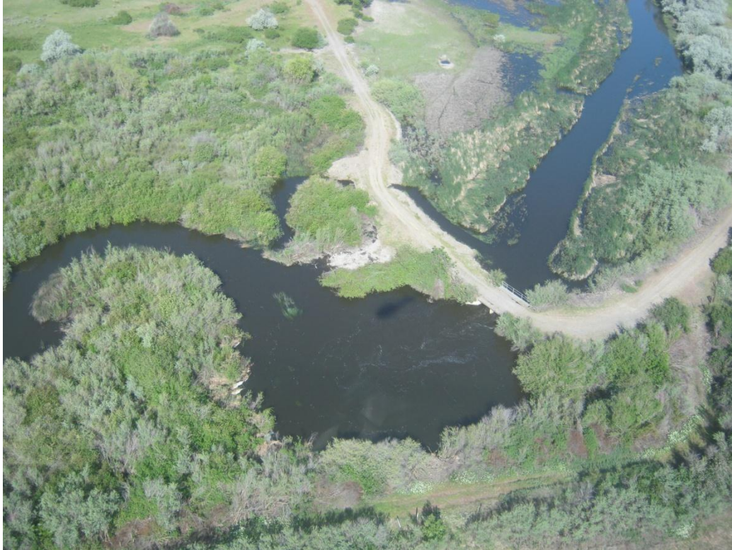
Figure 1. Durham Irrigation Dam (May 2011): Scour pool to the left (downstream) of the dam.
