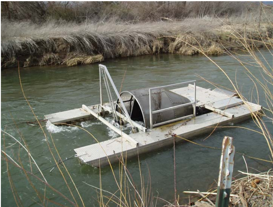
Figure 4. The five foot diameter screw trap deployed at Toppenish Creek.
